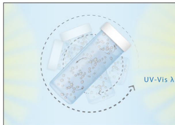
FIGURE 2 Illustration of the photoreactor with silica particles tumbling inside the vial
